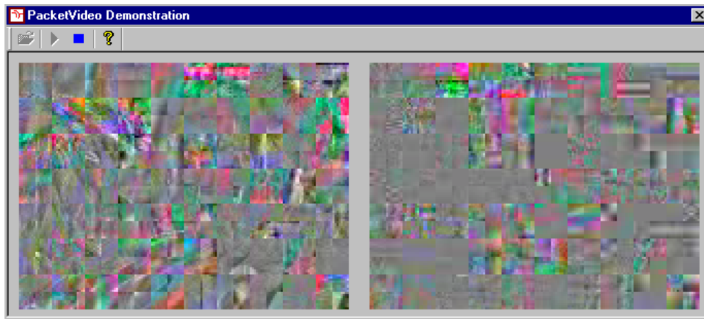
Fig. 7: Attacked frame of Fig. 6 by setting DCs of luminance component to 128, DCs of chrominance components to 0, and all MVs to 0.
